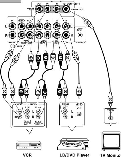
Connect phono cables from a VCR's audio outputs to the receiver's VCR/TAPE 1 or LD/DVD IN (audio) jacks. Then connect phono cables from the receiver's VCR/TAPE 1 OUT (audio) jacks to the VCR's audio input jacks.
